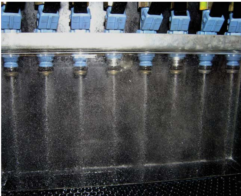
> On the test bench, you can clearly see the variation in fuel delivery volume.
