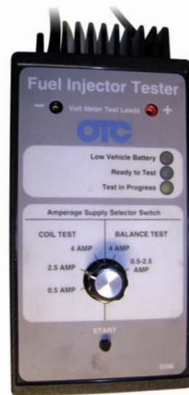
> This fuel injector tester will let you know if the actuating coil is shorted.
