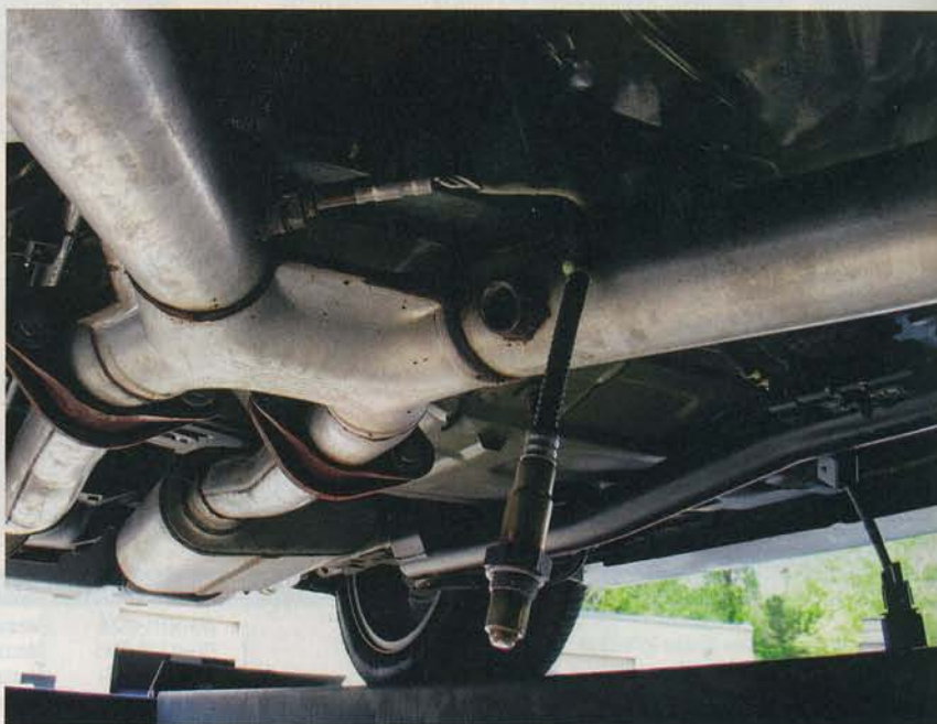
THE '04 Mustang we used as our subject vehicle was no longer using its rear O 2 sensors, so we utilized one of the available bungs to house the Bosch O 2 sensor supplied with the stand-alone gauge kit. The oxygen sensor must be connected and operating with the LC-1 whenever the car is running, as an unpowered oxygen sensor will be quickly damaged when exposed to hot exhaust gases.
