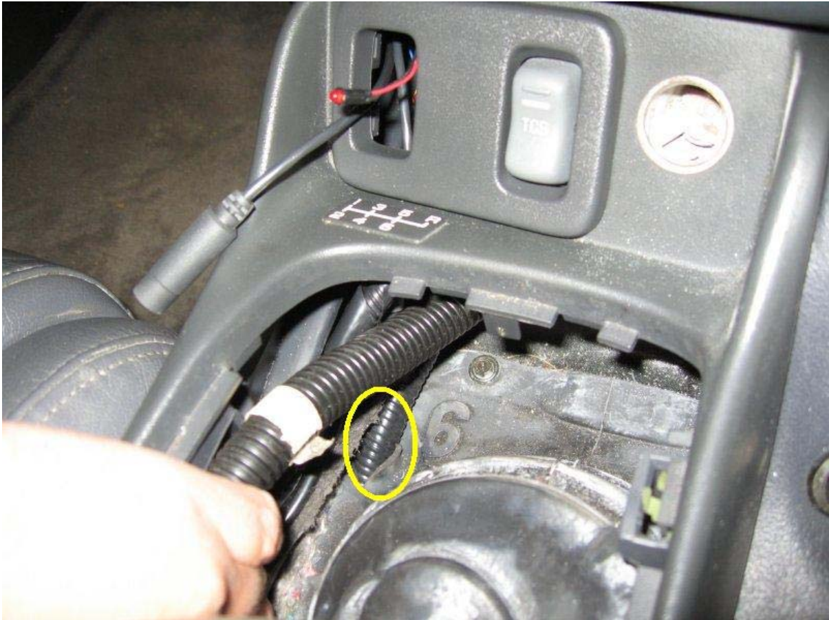
Picture 5: LC-1 Cable Routing (Cables in Wire Loom)
